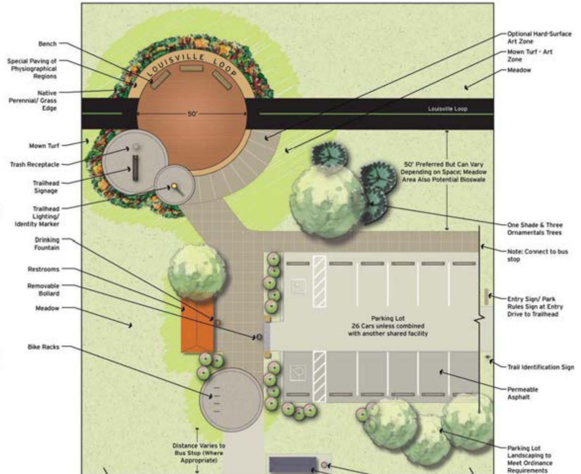
FIGURE 4-1: Prototypical Trailhead Design (from Design Standards Manual)
